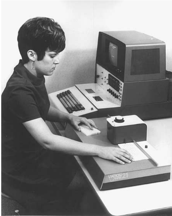
Figure 8.2 Office automation: Viatron 21. (Source: Charles Babbage Institute, University of Minnesota.)
